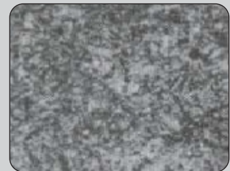
Untreated steel 1000x Magnified (right)
