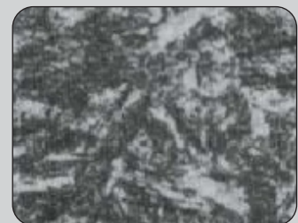
Cryo-treated steel 1000x Magnified (right) (Dark areas show formations of carbides)
