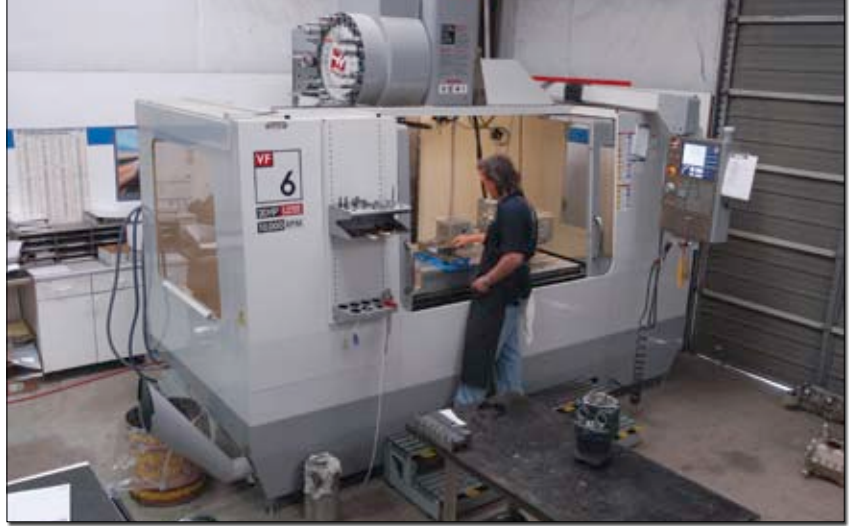
Ly-Con's 20-hp Haas CNC center is where the cutter meets the aluminum. The company is just beginning to explore the 2007 machine's capabilities; its speed and precision are rare commodities in general aviation engine work.
