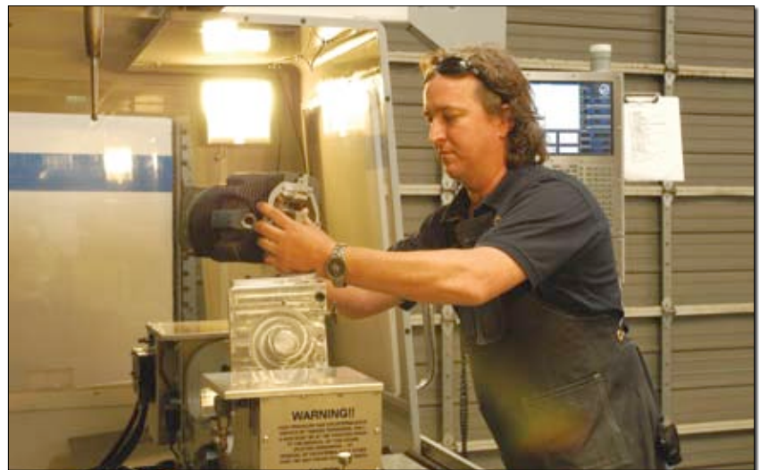
Ly-Con's 20-hp Haas CNC center is where the cutter meets the aluminum. The company is just beginning to explore the 2007 machine's capabilities; its speed and precision are rare commodities in general aviation engine work.
