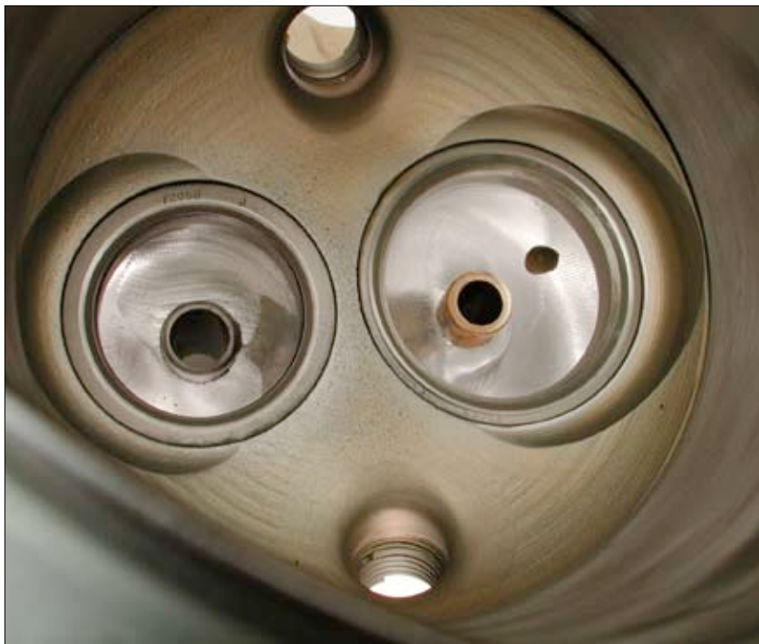
From the combustion chamber side the CNC ported head shows some registration lines in the smaller exhaust port, plus the opened area behind the bronze-colored valve guide in the intake port. No CNC work is done to the combustion chamber, nor have these valve seats been cut yet on the Serdi machine.
