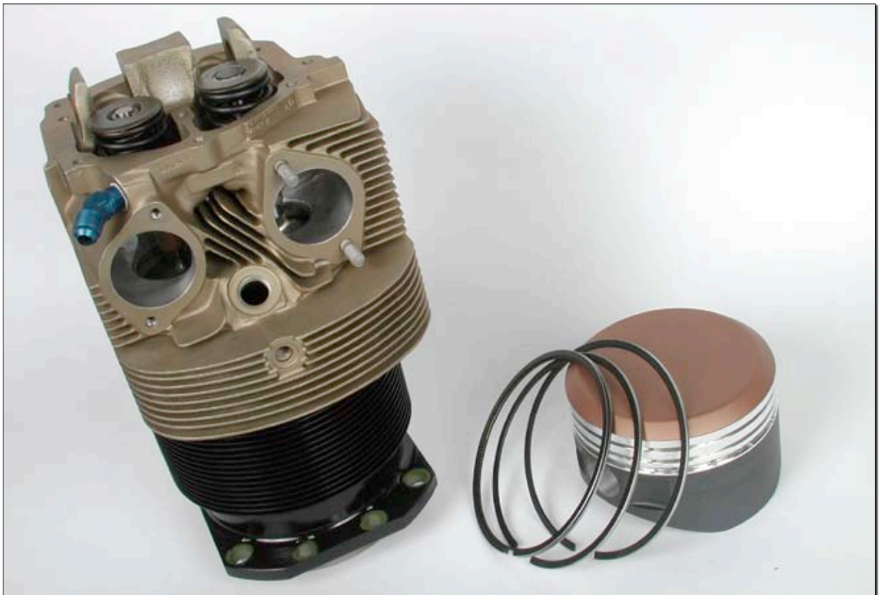
Ly-Con CNC ports Lycoming, Continental and Superior cylinders for certified and Experimental aircraft. Here a CNC-ported Lycoming 360/540 jug is matched with black cylinder paint, gold alodine anti-corrosion treatment on the head and a fully coated 10:1 NFS piston. With the higher compression, the combination is for Experimental aircraft only, but offers a real boost in performance and efficiency, plus some cooling and rust protection tweaks.
