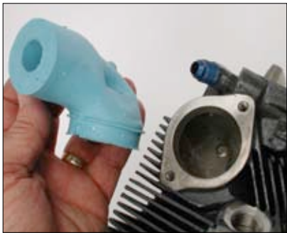
Writing CNC software is eased immensely if a male model of the port is available. Ly-Con formed the necessary molds with latex rubber, a common head-porting technique.
