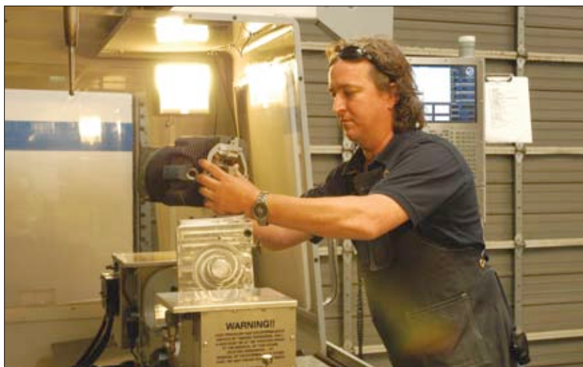
Ly-Con's 20-hp Haas CNC center is where the cutter meets the aluminum. The company is just beginning to explore the 2007 machine's capabilities; its speed and precision are rare commodities in general aviation engine work.
