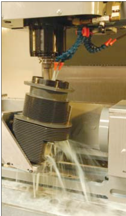
Replicating arm and wrist movement takes five-axis motion. The Haas machine does this with the usual three-axis table, plus a two-axis cradle bolted to the table. It's fascinating to watch the machine move the work in all five axes simultaneously. Essentially the cutter moves down the port in a carefully controlled spiral; access to both flange and cylinder apertures on the jug is easily accomplished.
