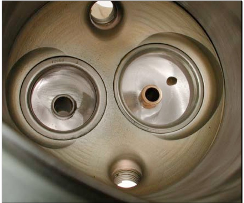
From the combustion chamber side the CNC ported head shows some registration lines in the smaller exhaust port, plus the opened area behind the bronze-colored valve guide in the intake port. No CNC work is done to the combustion chamber, nor have these valve seats been cut yet on the Serdi machine.
