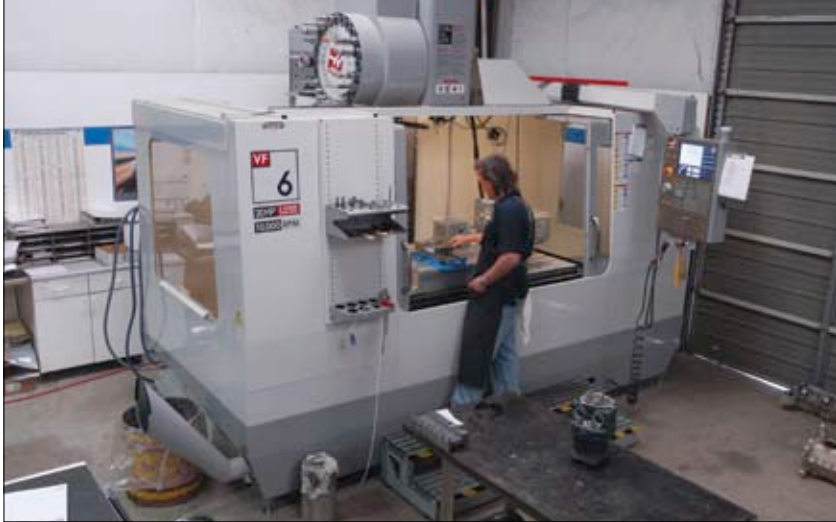
Ly-Con's 20-hp Haas CNC center is where the cutter meets the aluminum. The company is just beginning to explore the 2007 machine's capabilities; its speed and precision are rare commodities in general aviation engine work.
